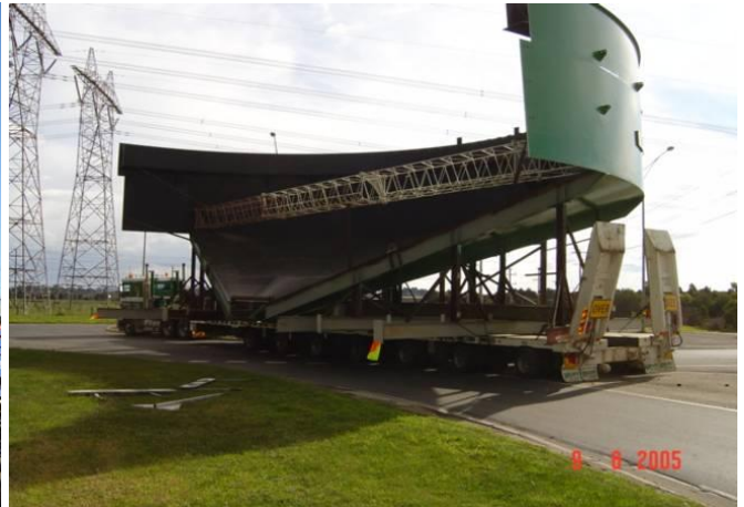
22m tank being transported to site
